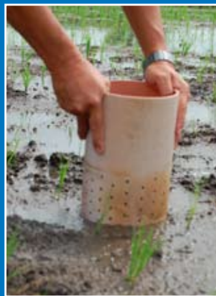
A SAMPLE field water tube made from polyvinyl chloride. Note the holes on all sides.
